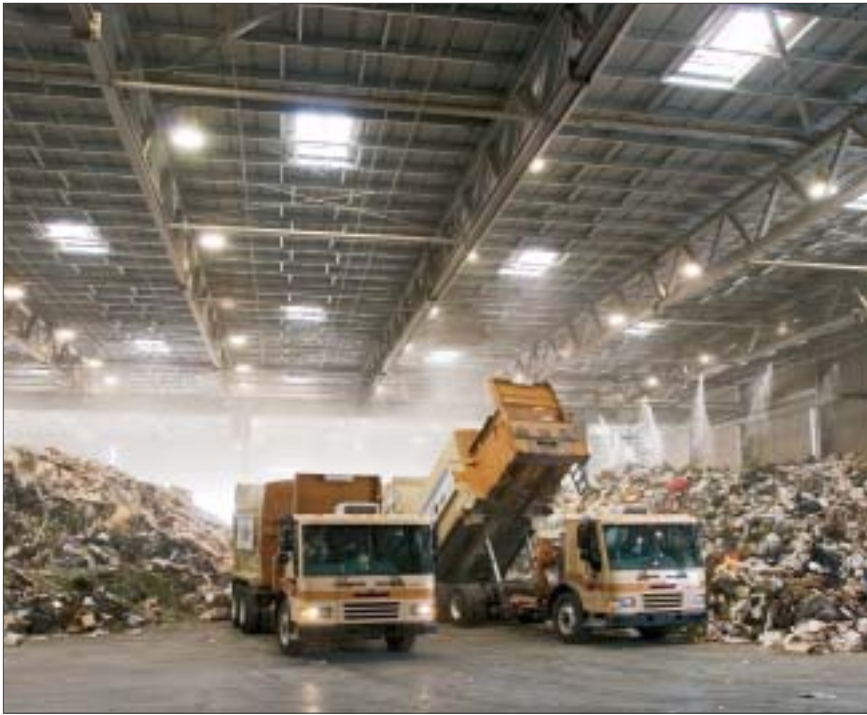
The tipping floor where route trucks unload collections that are reloaded into semis for the 60-mile haul to the new landfill.
