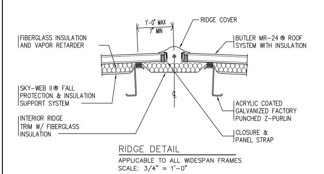
SECTION: Ridge WALL: ROOF: MR-24 STRUCTURAL: Widespan
